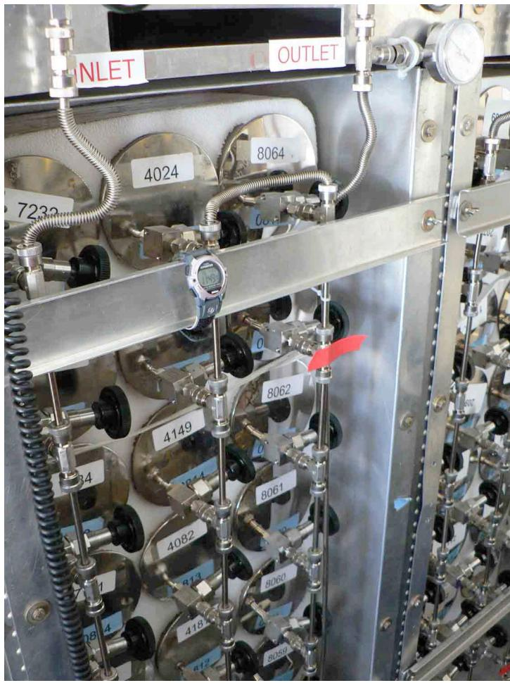
**Figure 1.** A UC-Irvine foam-embedded set of 24 linked, 2-L stainless steel samplings canisters installed on the NASA DC-8 aircraft during the TC<sup>4</sup> mission. Photo by Nicola Blake.
