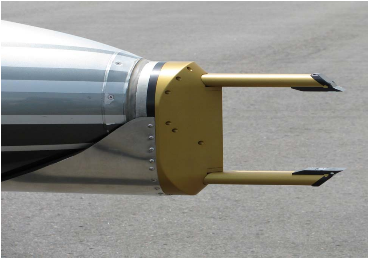
Photograph of SPEC HVPS probe installed in the PMS canister embedded in the tip tank of the SPEC Learjet.
