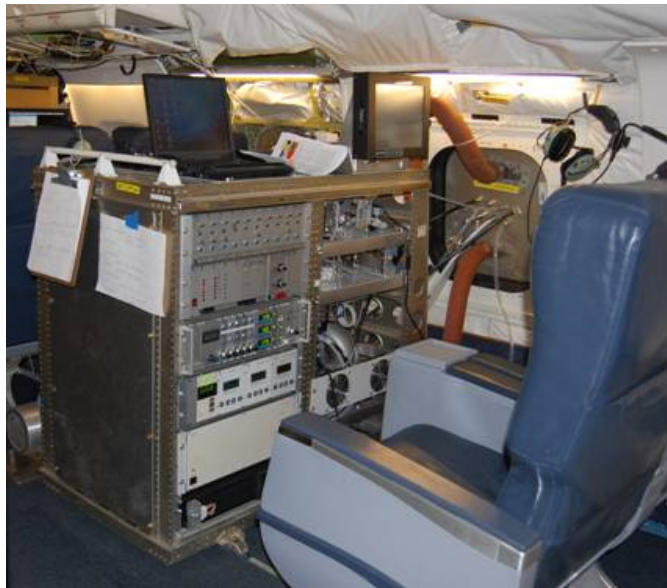
Figure 1: The Innsbruck PTR-MS instrument onboard the NASA DC-8
