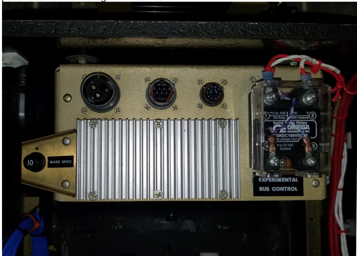
Figure 4 - Top view of Experiment Interface Panel (EIP), showing Vicor DC-DC converter under heat sink.
