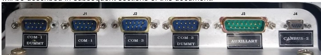
Figure 5: Top view of Auxiliary Interface Panel (AIP) and D-subminiature connectors. The AIP features a number of RS-232 ports, dummy jacks to permit parking of avionics cable plugs when not in use, and facilities for straightforward routing of payload cables to the AIP and fixing them in place.
